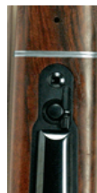
Lever is returned home and locked. The rifle is now ready for use.
